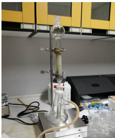
Fig. 5: Column chromatography of the crude extracts
