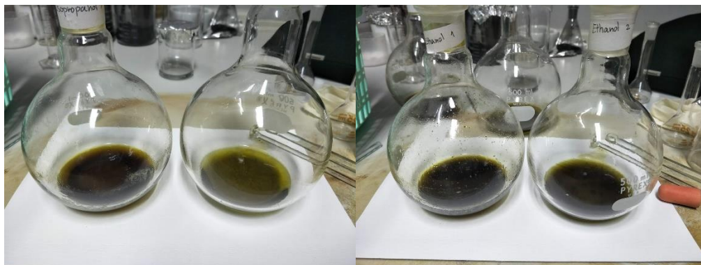
Fig. 2: The crude extracts of cannabis using EtOH (a) and iPrOH (b) as the extractants.
